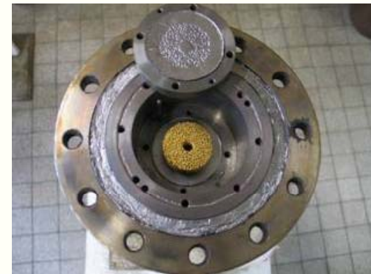
Catalytic Sponge Reactor for Gas Purification Processes
